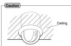
Embedded Cover in Ceiling (recess bracket)
